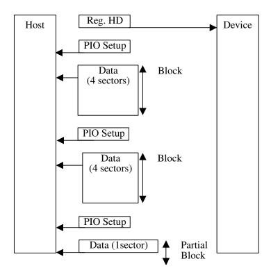
Figure 5.12 Execution example of READ MULTIPLE command
